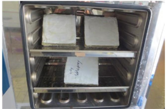
Climate chamber used for the aging test
